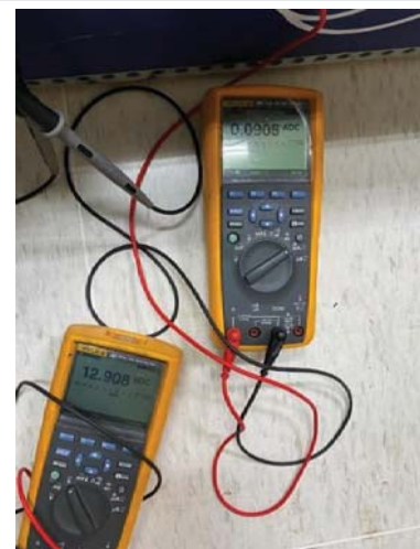
Figure 6: Using Handheld Digital Multimeters to measure the Aquadopp-6000m Current meter. While recording, the current and voltage at the battery terminal are 0.0908 A and 12.908 V, respectively. Credit: Ching-Ren Lin.
